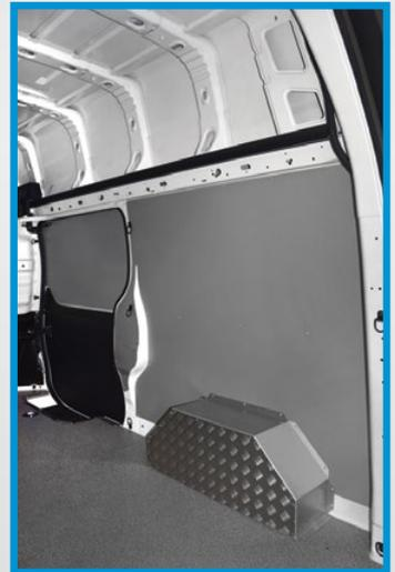
**Vivaro/Trafic 2014/Talento 2016/NV300 H1:** Floor liner in marble-look beech plywood, bodywork liners in grey pre-painted steel sheet, wheel arch covers in aluminised steel sheet and aluminium tread plate
