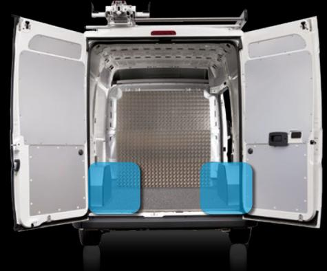
Syncro can protect your van's wheel arches too. Syncro wheel arch liners consist of an upper section in 2 mm thick pre-shaped aluminised steel sheet and a vertical side in marble-look or rubber-coated plywood or in aluminium chequer plate.
