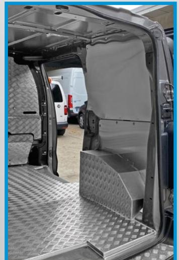
**Expert/Jumpy/Proace 2016/Vivaro 2019/Scudo 2022 L2 H1:** Double-layer floor liner in 9 mm birch plywood and aluminium tread plate, bodywork liners in aluminium, bulkhead liner in aluminium tread plate, wheel arch liners in aluminised steel and aluminium tread plate
