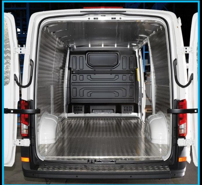
Liners are available for the roofs of most vans, and customers can choose from versions in prepainted steel, anodised aluminium, honeycomb polypropylene or aluminium tread plate.
