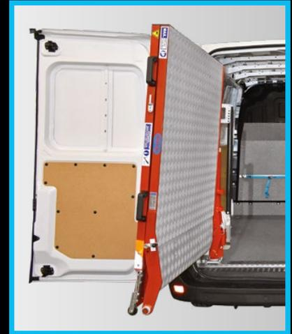
Ramp pivots to one side for easy access to the cargo compartment
