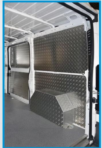
**Ducato/Boxer/Jumper 2006/Movano 2022:** Floor liner in marble-look beech plywood, bodywork and bulkhead liners in aluminium tread plate, wheel arch covers in aluminised steel sheet and aluminium tread plate
