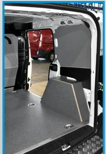
**Doblò 2010/Combo 2012:** Floor liner and bulkhead liner in marble-look beech plywood, wheel arch covers in aluminised steel sheet and marble-look plywood, bodywork liners in grey pre-painted steel sheet
