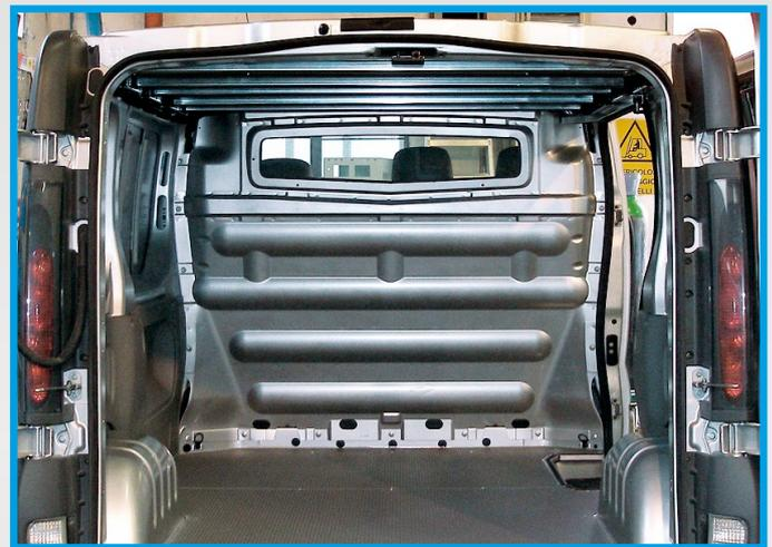
Syncro hanging garment bars incorporate a spring-loaded fixing system that engages quickly and easily in holes in the accompanying rails. The rails can be positioned wherever you need, so that you can exploit the space in your van in the most efficient way possible.
