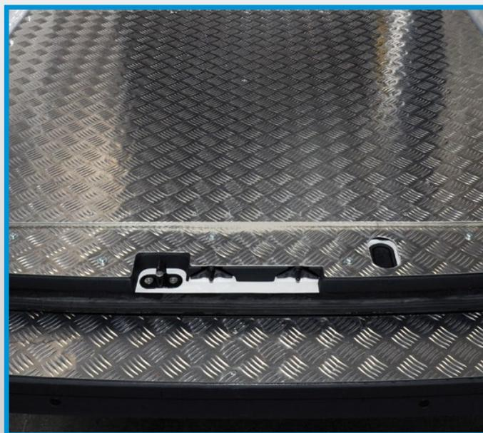
These products in aluminium tread plate protect the top of the bumper against impact and wear and provide a robust, non-slip surface for climbing into the cargo compartment.
