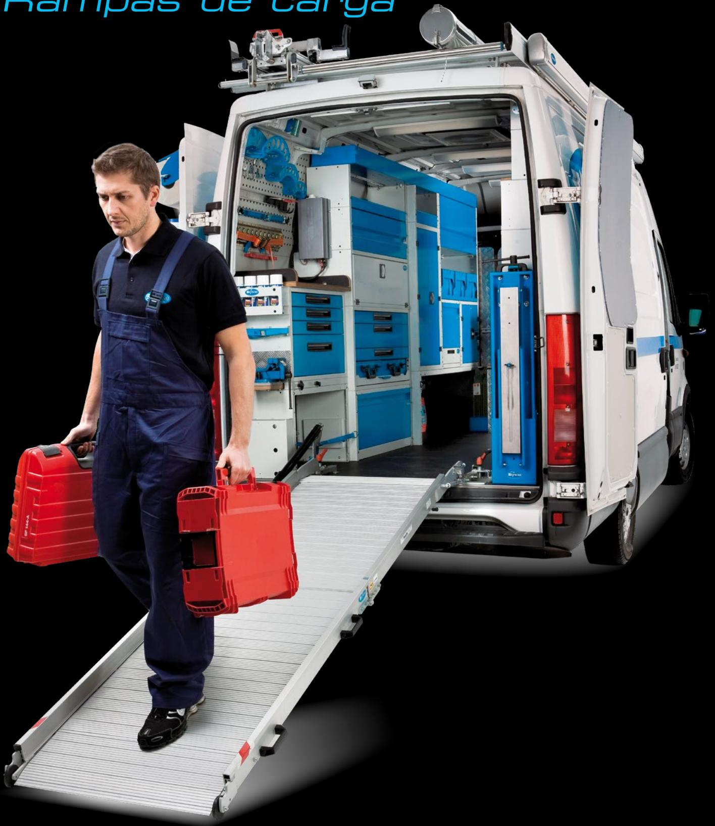
Syncro System loading ramps make safe and easy work of loading and unloading even heavy items. They can be extended and lowered to the ground with only minimum effort, thanks to gas springs that support the weight.
