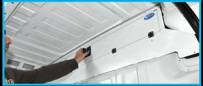
These practical storage units use a high-strength steel sheet to enclose the space at the top of high-roof cabs and create secure and functional storage. The space created in this way is accessible via a lockable, double-latch door. Security is ensured by a lock with key. Quick and easy to install. There is never enough room in the van, but these clever storage units let you make the fullest use of what space there is!
