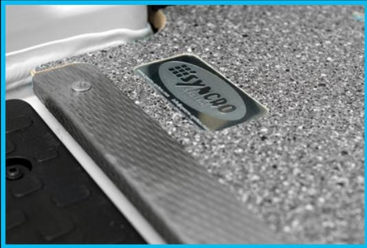
Syncro plywood floor liners come with stainless steel edge protectors for use at the doors. These tough protectors prevent damage to the liner during loading and unloading. Edge protectors also come cut to size and ready for installation. Their non-slip surface conforms to current safety standards. Edge protectors are included in the price of Syncro floor liners, but they can also be purchased separately and used with non-Syncro floor liners.
